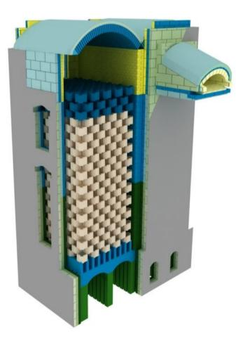
Alumina Chrome, Magnesia, Mag-Zir Chimney checkers block with new design for Regenerators application for Energy savings solution due to large heating surface, high heat transfer and low tendency of blocking and clogging.
